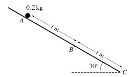
Three points A, B and C lie on a line of greatest slope of a plane inclined at an angle of  $30^{\circ}$  to the horizontal, with AB = 1 m and BC = 1 m, as shown in the diagram. A particle of mass 0.2 kg is released from rest at A and slides down the plane. The part of the plane from A to B is smooth. The part of the plane from B to C is rough, with coefficient of friction  $\mu$  between the plane and the particle.
