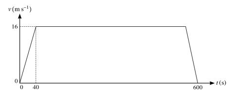
The diagram shows the velocity-time graph for a train which travels from rest at one station to rest at the next station. The graph consists of three straight line segments. The distance between the two stations is 9040 m.
